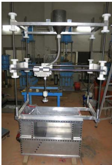
Fig. 5 Sand pluviator on the fault simulation container
