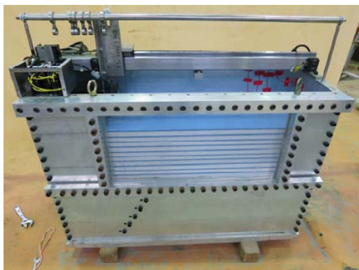
Fig. 1 Fault simulation container
