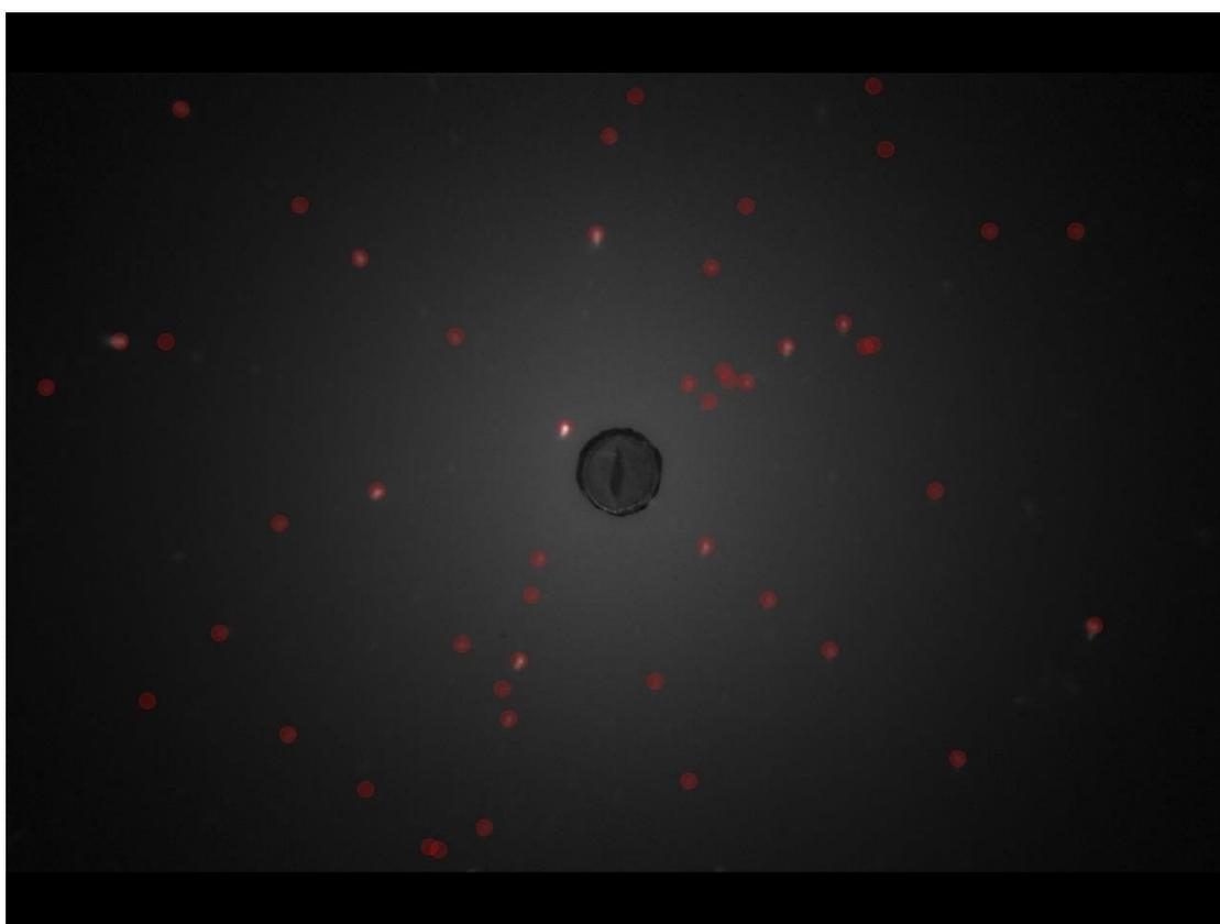
Figure 5. Picked points from the Laue-diffraction pattern of  $c$ -axis.
