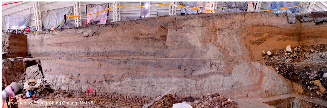
Figure 15. North walls of the Chushan trench in 2005 and 2012. (a) Photograph (left) and cross section of structures (right) of the 2005 north wall. The peeling project was ongoing while the photograph was taken. (b) Cross section of structures (up) and photograph (down) of the 2012 north wall. The dashed box circles an area which might be affected by post-earthquake effect attributed to an excavator (at middle left in Figure 8a).
